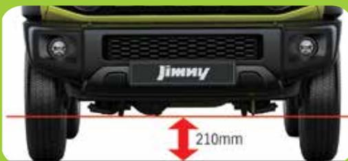
Ground clearance has been increased to 210mm (+10mm) to provide enough height to tackle even the toughest terrain.
